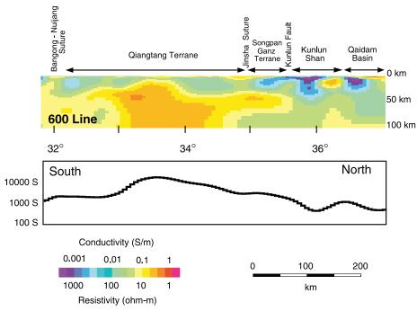
Fig. 3. Electrical conductivity model for northern Tibet (600 line).
