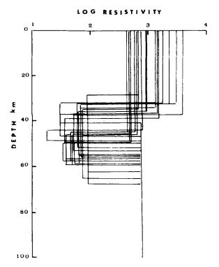
Figure 7. The resistivity-depth profiles for PRE rotated major data at the 94 per cent acceptance level.
