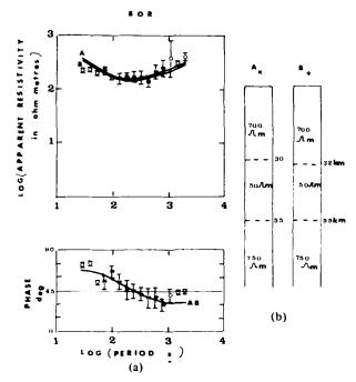
Figure 1. (a) The apparent resistivity and phase data for BOR – the asterisks denote well-estimated values and the open circles the other values. (b) Electrical conductivity models A and B – the initial and final models of the Monte-Carlo inversion of the BOR major data. The theoretical apparent resistivity and phase curves are drawn in (a).
