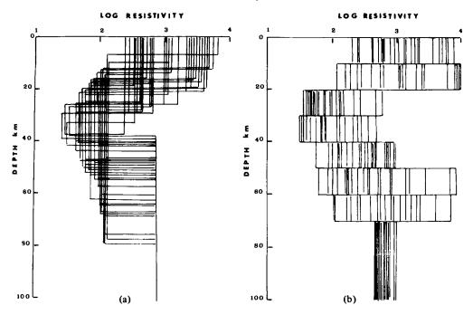
Figure 6. The resistivity-depth profiles for NEW rotated major data at the 90 per cent acceptance level. (a) 3-layer models. (b) 8-layer models.
