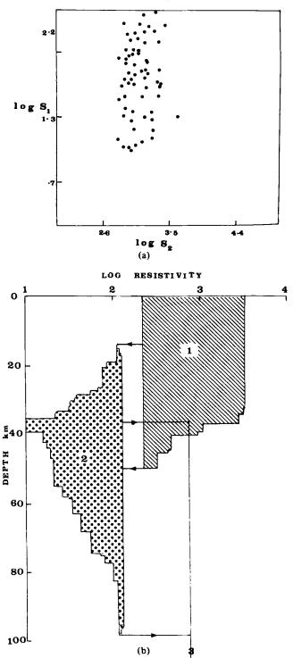
Figure 3. (a) The S-space for the Monte-Carlo inversion of data from BOR at the 85 per cent acceptance level. (b) The resistivity-depth profiles of models acceptable to the BOR responses at the 85 per cent acceptance level. For clarity in this diagram, the outermost bounds only for the three layers have been indicated.
