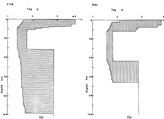
Figure 5. (a) Outline of resistivity-depth profiles for ITH rotated major data at the 80 per cent acceptance level. (b) Outline of resistivity-depth profiles for SAL rotated major data at the 75 per cent acceptance level.
