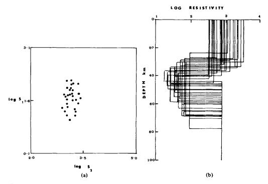
Figure 4. (a) The S-space for the Monte-Carlo inversion of data from BOR at the 94 per cent acceptance level. (b) The resistivity-depth profiles of models acceptable to the BOR responses at the 94 per cent acceptance level.
