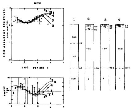
Figure 10. A comparison of 3 and 4 layer theoretical models for NEW. The apparent resistivity and phase curves for each of the models (b) is superimposed on the apparent resistivity and phase values plotted in (a). The model depths are in kilometres and resistivities in ohm metres.
